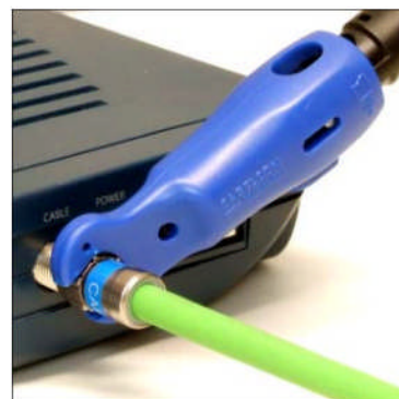
Proper tightening with the Pocket installer
