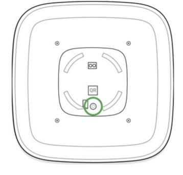
The on/off button is recessed into the body of the siren and quite tight, you can use a thin solid object to press it.
