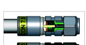
CX3™ QuickMount™ is equipped with Cabelcon's unique PushPin™ system (patented) for a safe grip on the inner conductor and easy determination of properly inserted cable. The pin is visible when the cable is in place!
