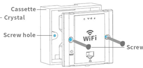
3.Match the AP and cassette through the screw hole ,and plug in screws to fix it, please do not make the screw too tight.
