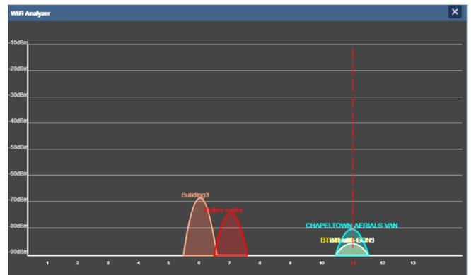
**2G and 5G WiFi:-** Setup the SSID (Name of the WiFi), Bandwidth, channel, Encryption and password. This area also has a built-in WiFi analyser to look for the best channel to set the 2.4/5G signal so that it doesn't clash with other channels.
