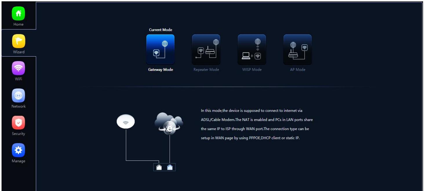
**Gateway mode:** - The AP will allocate IP numbers to the connected devices. This mode is default as it permits you to connect and setup the AP very easily.
