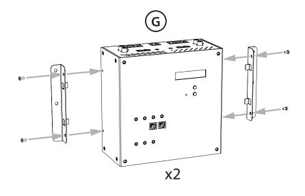
3. Mount each NetAmp onto rack panel using screws provided (4 screws per NetAmp).
