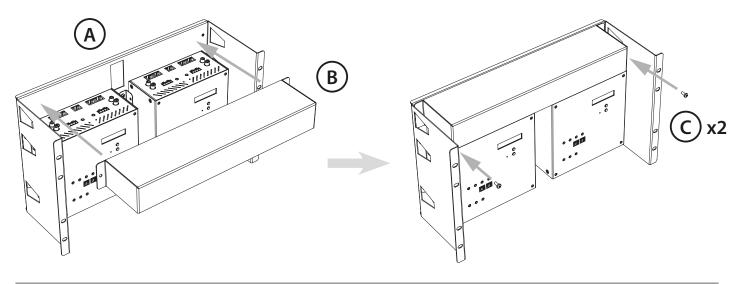
6. Fit 8 cage nuts into appropriate positions in the rack. Fix rack panel into rack using 8 screws provided.
